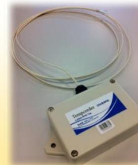
Different from most active RFID tags, **Extreme Tag** is equipped with an external probe which detects temperature range from -200°C to +500°C. When used to measure temperatures in extreme conditions, the probe will be placed in contact with objects that are extremely hot while the body of the tag remains at another location which is of less extreme temperature. The smart design enables temperature control for a wide variety of areas, especially suitable for places where are dangerous for human.
